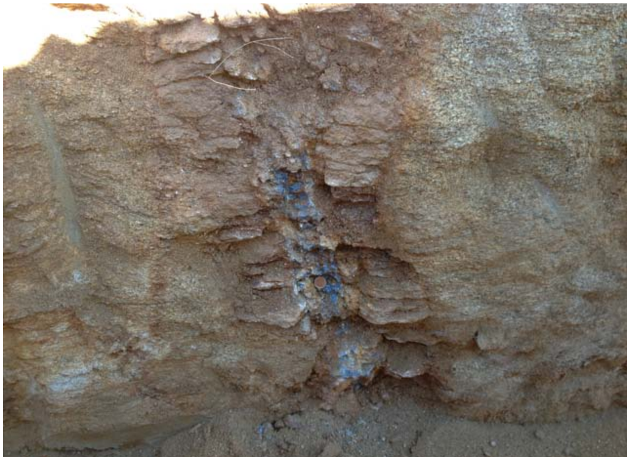
Gold-bearing quartz-sulphide vein in trenching at Cabeza de Caballo
